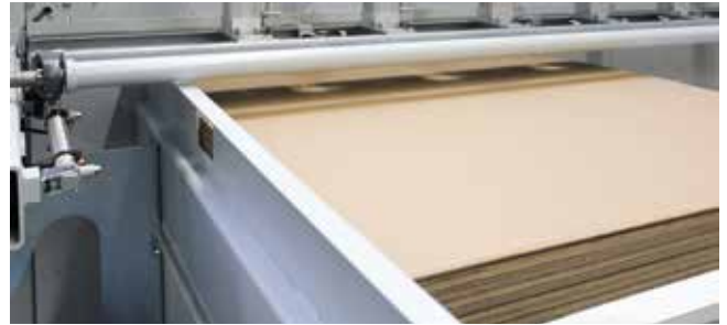
The automatic single-sheet feed with lifting table enables the automatic supply of stacked single-sheet materials.
