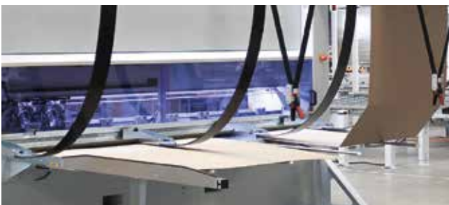
The combination cardboard box supply enables the supply of single sheets as well as the use of continuous cardboard.
