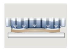
Pressure and compensation behaviour of the individual segments for warped workpieces or workpieces with thickness tolerances. Within the tolerance range of max. 2 mm the same pressure is applied to different areas of the workpieces.
