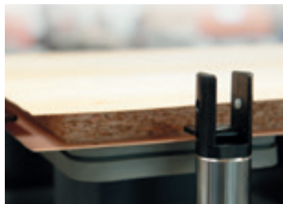
Stop pin for covering layer overhang with end position monitoring to protect tools, units and machine operating personnel
