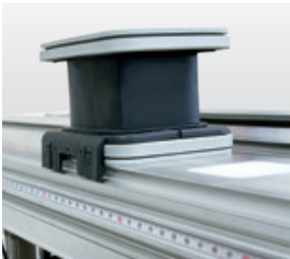
Measuring tape for positioning the suction units.
