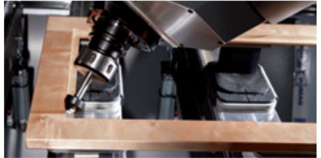
Square corner cutting for a glass rebate
