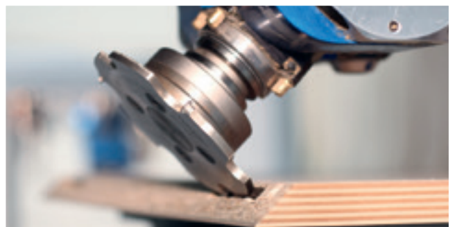
Cutting recesses for connecting fittings
