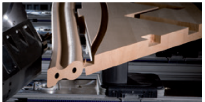
Holes for piling at narrow angles
